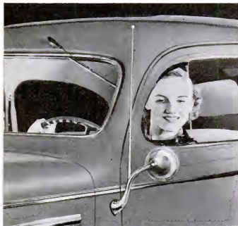
The mirror back and bracket increase the pick-up area
